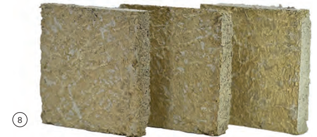
fig. 8 "Phragcrete" modules utilized phragmites hurd and hydrated lime (derived from shellfish waste), allowing Jais to form this material completely from maintenance waste and food waste.
